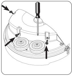
Attach Right Hand Brush Deck Cover using 3 screws and washers at the fixing points shown above.
