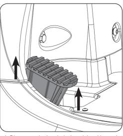
Disengage the brush deck pedal and lower the brush deck.
