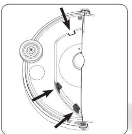
Locate the Left Hand Brush Deck Cover on to the Left Hand side of the brush mount. Make sure the elbow fitting is fully located under the cover of the brush deck.
