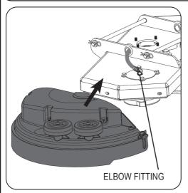
Locate the Right Hand Brush Deck Cover onto the Right Hand side of the brush mount. Make sure the elbow fitting is fully located under the cover of the brush deck.
